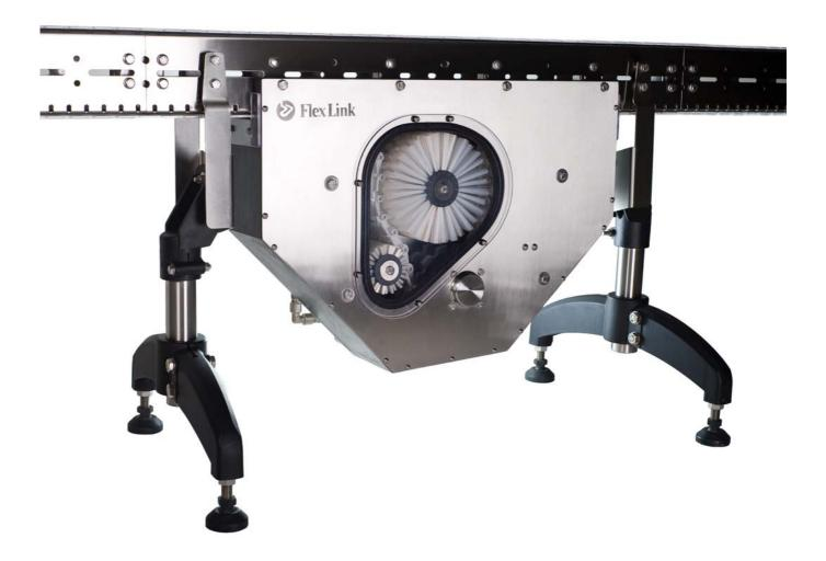
The inline chain washing unit is designed to run continuously when working with production lines that have a high degree of product spillage. The result is a cleaner chain that allows longer production runs without the need for CIP or routine maintenance.
