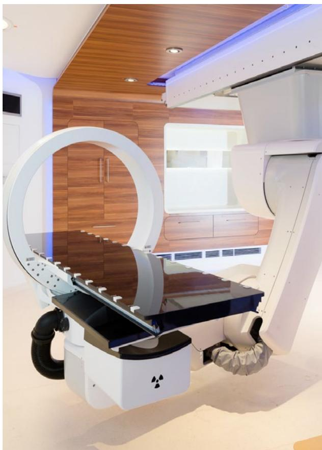
BEC uses KUKA robots for precise positioning of the patient during particle-based radiation therapy (© Thomas Kästenbauer)
