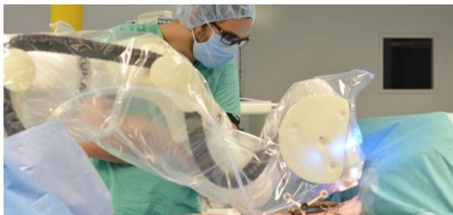
The laser head – held by a KUKA LBR – enables bone surgery to be performed with unprecedented precision (© AOT)
