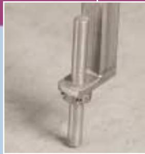
The infinitely adjustable floor-foot design provides point contact with the floor. Combined with sealed construction and a non-threaded rod, the design simplifies sanitation and maintenance.
